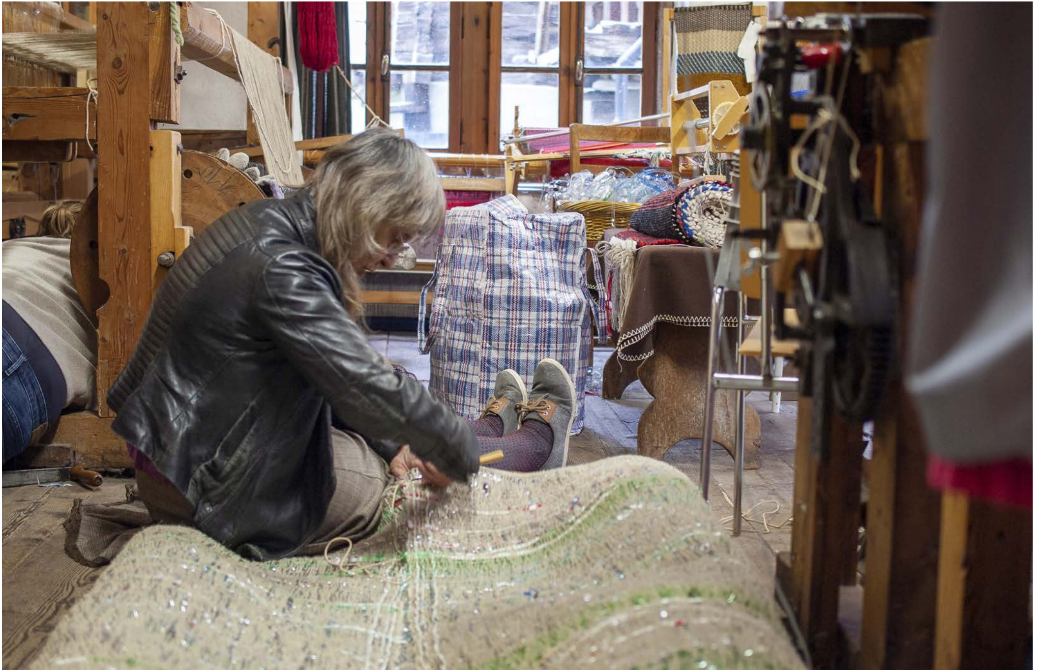
Manufacturing of the second carpet woven with PET and cannabis yarn, Atelier Marie Metrailler, Evolène, 2019
